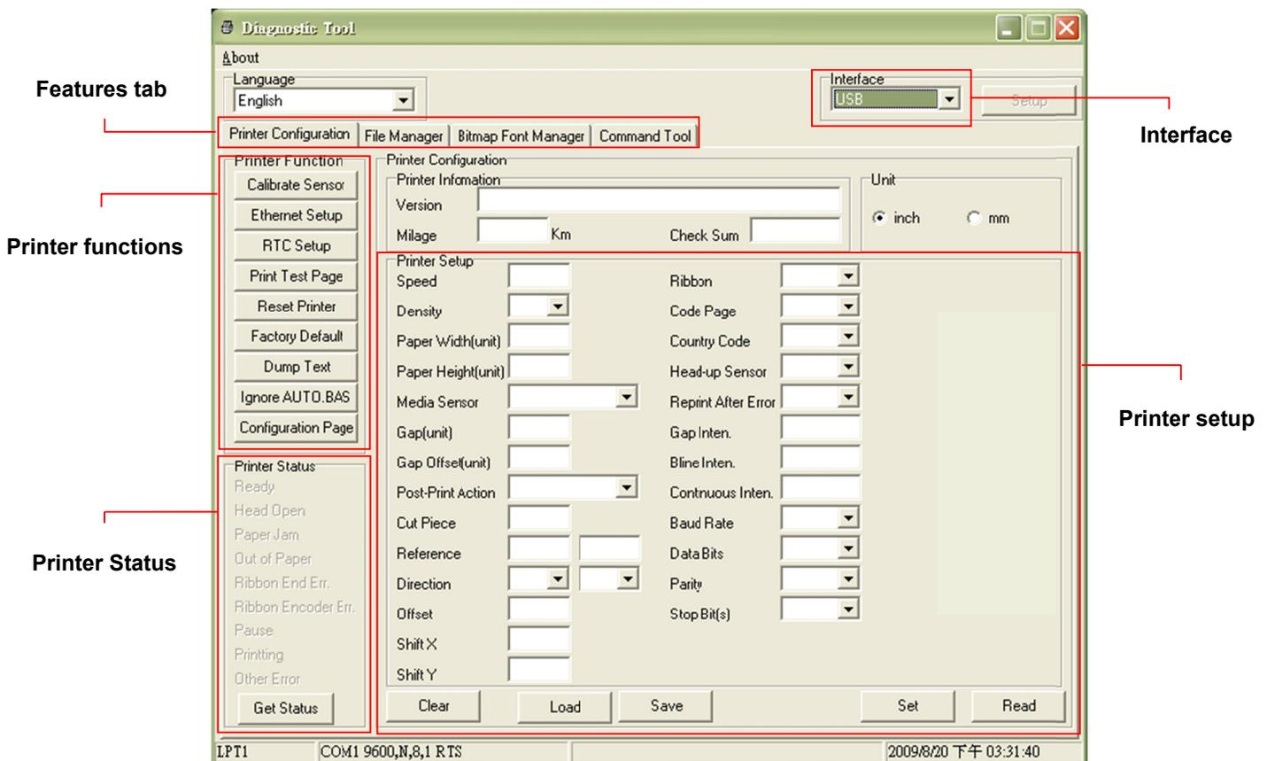
**3.3.2 Printer Function (Calibrate sensor, Ethernet setup, RTC setup.....)**
