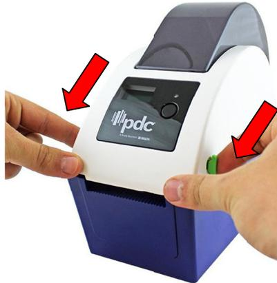
3. Separate the media holders to the wristband roll width.
